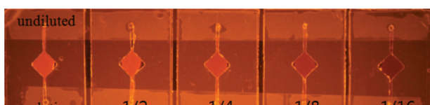
FIGURE 12. The reference plate image captured by the conventional 4 lamp UV illuminator
